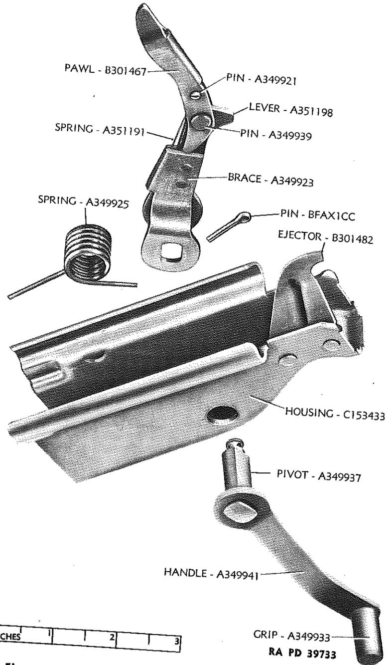
Figure 7 - Housing Group Parts for Gun, Submachine, Cal. .45, M3
