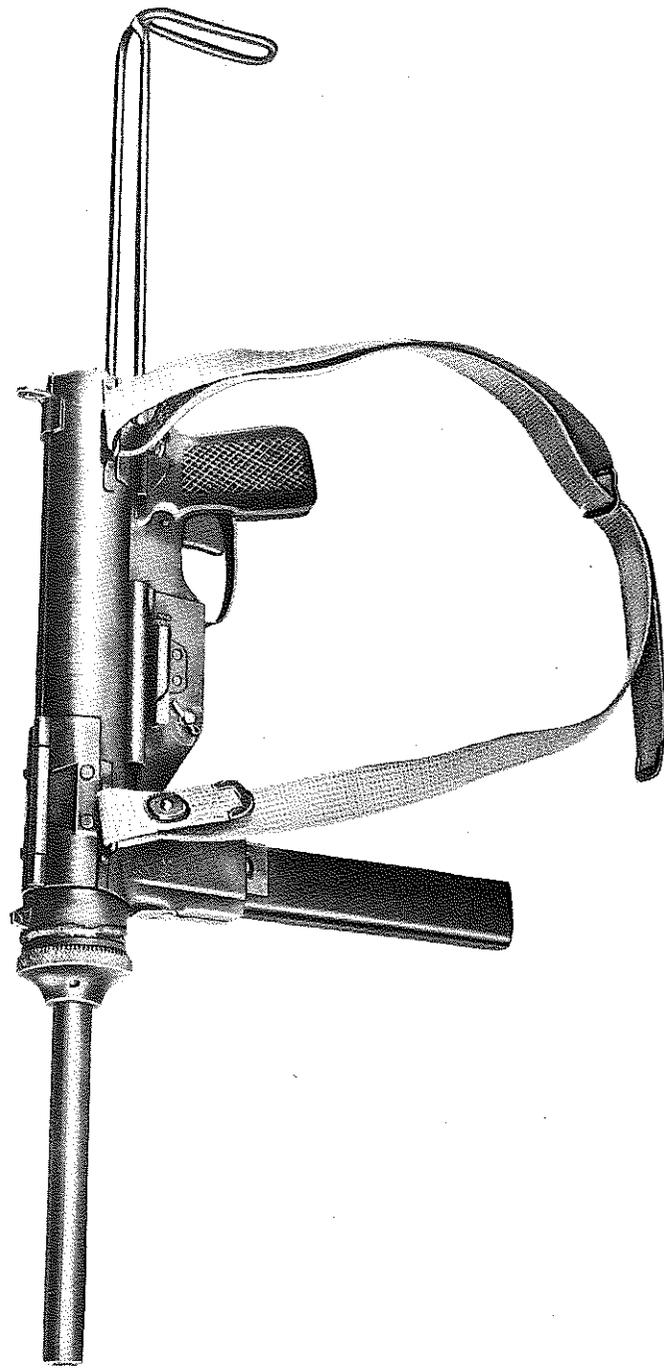
Figure 2—Submachine Gun, Cal..45, M3—Left Side View
